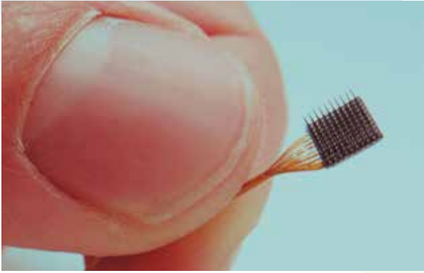
Blackrock Neurotech's Utah Array is a 4.2 millimeter square grid with 100 silicon electrodes.
